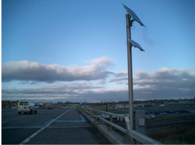
IR Laser Beam is focused on Bridge Deck Surface.
